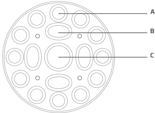
**A** Connection holes | **B** Connection eyelets | **C** Anchor hole
