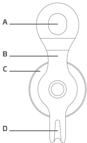
**A Main connection hole | B Flange | C Sheave | D Secondary connection point**
